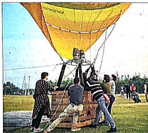
The baskets are connected to ropes, which will be tied to the ground for safety.
